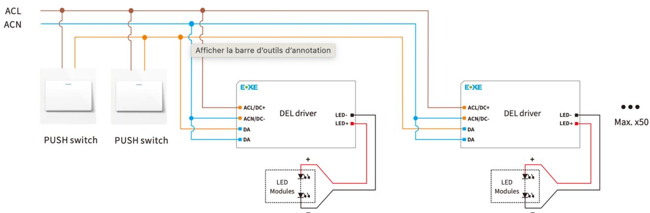
METTRE SOUS TENSION ET APPUYEZ 15 SECONDES SUR LE BOUTON POUSSOIR AINSI TOUS LES LUMINAIRES SE REGLERONT A 100% D'INTENSITE. APPUIE COURT = ALLUMAGE / EXTINCTION. APPUIE LONGUE = VARIATION.
